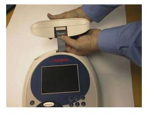
4. Plug the accessory cable into the printer.
