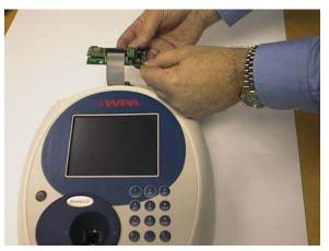
3. Plug the accessory cable into the Bluetooth module.
