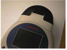
5. Lower the printer onto the locating bosses and push down firmly.
